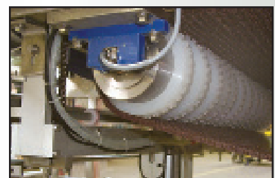
Motorized Pulleys Replace Greasy Chains
