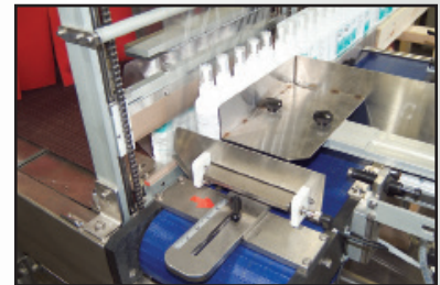
Fast Tool-Less Changeovers with Scales and Adjustable Handles
