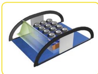
Film Cut from the Supply Roll
