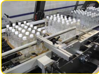
Tray Forming and Loading Section
