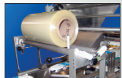
Film Cradle for Easy Film Loading
