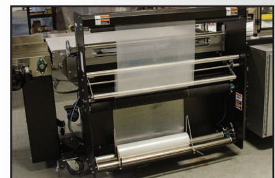
Side Mounted Film Cradle for Easy Film Loading
